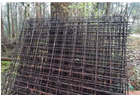
Reinforcing Steel Mesh
