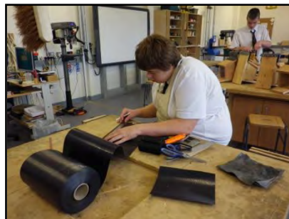
Danny cutting new, flexible hinges from a roll of dampcourse.
